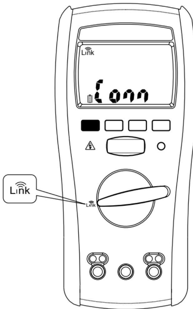
The meter uses Bluetooth low energy (BLE) V5.0 wireless technology to download the stored data. The open-air communication range is up to 6m. The LINK icon of the meter will freeze on LCD after the connection establishes successfully.
