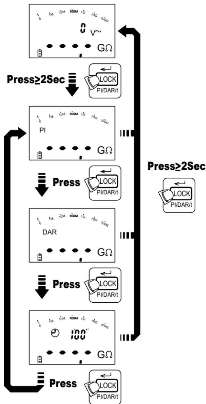
Press TEST button to start/interrupt the PI/DAR test.
