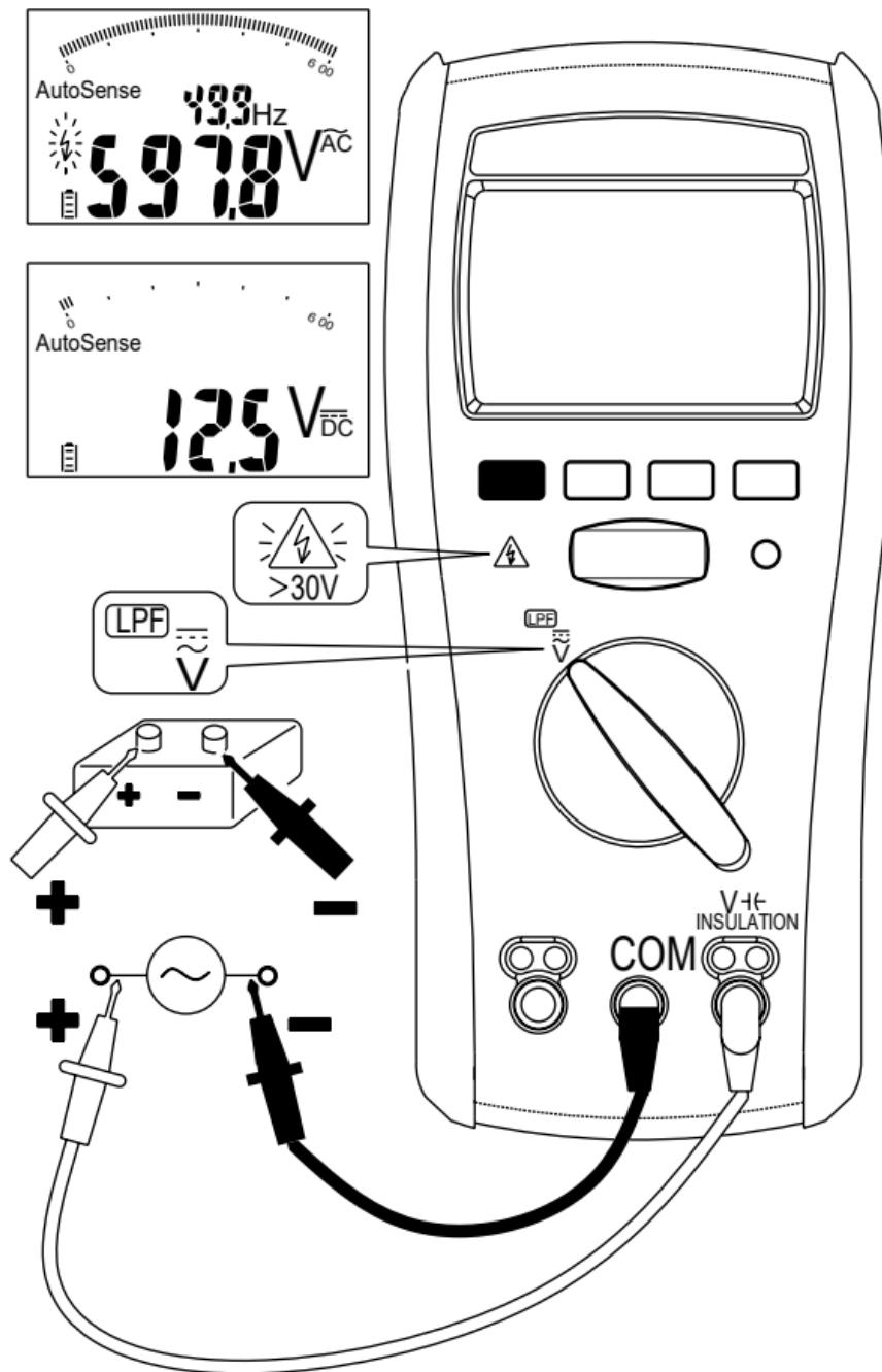
Auto sense mode: The meter displays ACV or DCV whichever is higher (>1V).
