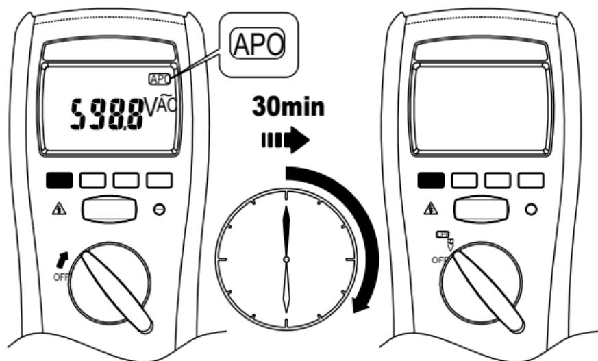
Restore power by switching rotator or by pressing any button.
