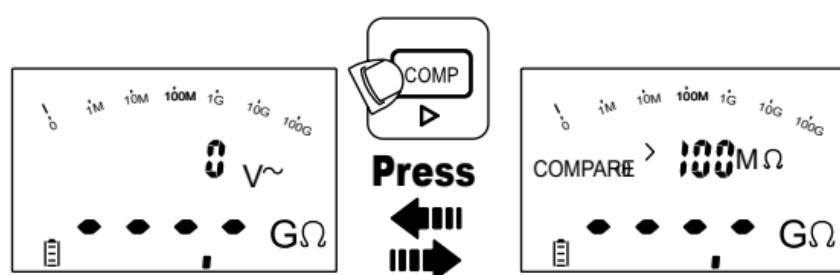
Before starting the Insulation Resistance test, select the comparative value in Setup mode:  $0.5\Omega$ ,  $10\Omega$ ,  $20\Omega$ ,  $50\Omega$ ,  $100\Omega$ ,  $200\Omega$ ,  $500\Omega$ ,  $1000\Omega$ .
