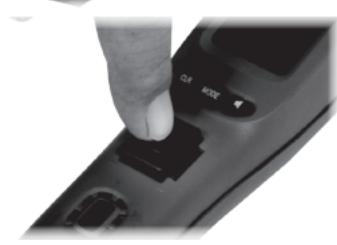
Position the new Rocker Switch into the switch cavity and carefully press straight down until the switch is flush with the housing.
