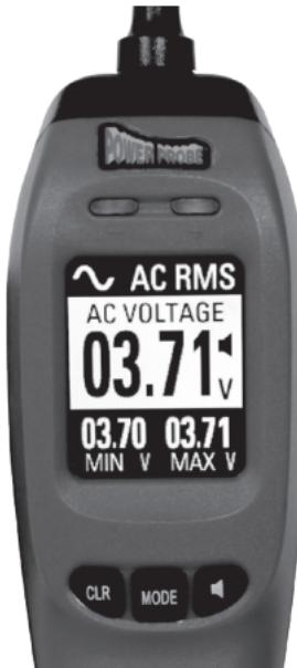
Contact the probe tip to the circuit and it will display an RMS averaged AC voltage reading in the main display area while also displaying RMS Min/Max AC voltages on the bottom line.
