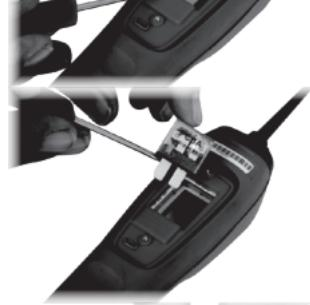
Once the Circuit Breaker is loose from the terminals, carefully lift the breaker from the housing cavity.
