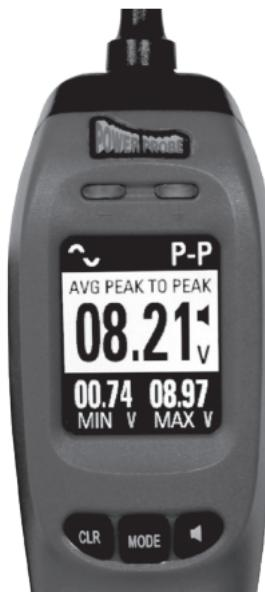
P-P stands for Peak to Peak AC voltage. Where AC RMS displays an averaged AC voltage, P-P does not average the reading but displays the total voltage difference from the lowest to highest voltage extreme on an AC signal.
