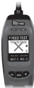
Pressing the rocker switch in any other mode will not apply power or ground and the main screen will display a large red "X".
