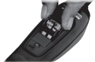
Position the new Circuit Breaker into the housing, take care to line up the breaker spades with the breaker terminals, and press down gently until the Circuit Breaker is fully engaged into the breaker terminals. Replace the rear cover and the two retaining screws.
