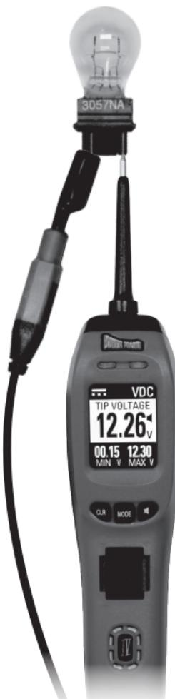
Activating Electrical Components in VDC Mode is one of the main features that make the Power Probe IV very useful when testing. Being able to apply battery power or ground right to the probe tip gives you the ability to activate and dynamically test electrical components such as lights, motors, and solenoids.
