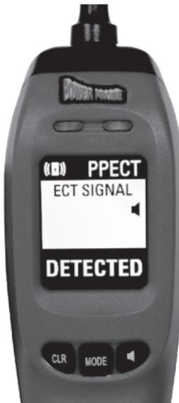
When using the ECT2000 to find opens in wiring, the ECT Transmitter injects a specialized digital signal that is normally picked up by the wireless ECT Receiver. In some situations, such as large wiring bundles or limited access, pinpointing the ECT signal and locating the exact point of the wire failure may be difficult when using the ECT Receiver alone.
